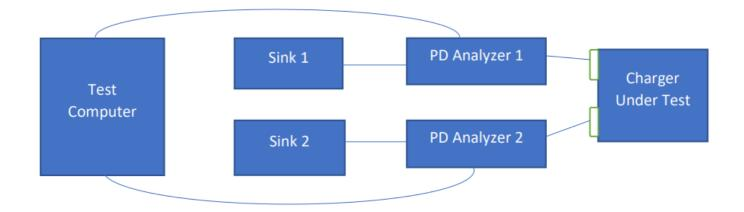
Some PD Analyzers, such as the GRL A1, can have multiple recording instances on one test machine as assumed in the setup shown above and the test procedure described below. Note that if the PD Analyzer used for testing needs one host machine for each PD Analyzer capture, such as for the Total Phase PD Analyzer, the test setup and procedure must be modified to include one Test Computer for each PD Analyzer.
