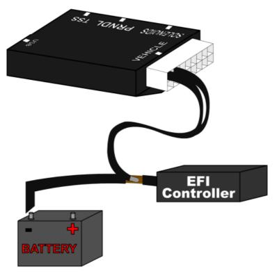
We often say that the ground is the most important connection you will make when installing our transmission controllers and this statement is especially true when using one of these EFI systems. Since the two systems are sharing a critical signal input, they must be at the same ground potential. Both of the black ground wires from the Quick controller must be connected to the main ground of the EFI system, as close to the EFI ECU as possible.
