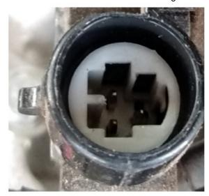
If there is a white or gray insert in the connector, use needle nose pliers to remove it.
