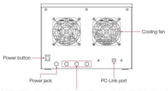
Additional Power jacks for use with USB-HDDs on duplicators with 16 or more ports.
