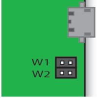
To reset the unit the jumper W1 must be open, as shown in picture. Insert a new bag and push metal connector till a "click" is heard.
