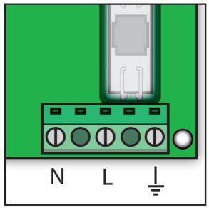
While connecting the machine to the mains power, it is recommended to pay attention to the connection and the screwing of the terminal block screws. The fact of disconnecting or modifying the ground cable voids the warranty and can cause troubles or accidents related to the temperature control.
