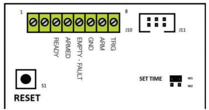
To set the shooting time, after opening the front panell, you must close the jumper W1 in SET position as shown in figure, then, holding down the button S1 "RESET", the green led on the front will flash and each flash is equivalent to one second. If you press the button again, the shooting time is not added to the one previously set, but will restart from zero.
