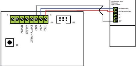
The ON/OFF output of this alarm panel is an Open Collector NPN that is OPEN with the alarm OFF and close to negative for all the time the alarm panel is active and monitoring. The alarm panel output is normally open and close the contact during alarm time.
