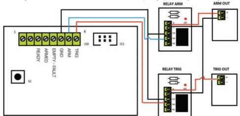
The ON/OFF output of this alarm panel is an open relay when panel is OFF that continuously keep close for all the time the alarm panel is monitoring. The alarm output of the panel is an open realy that close when alarm condition is detected.
