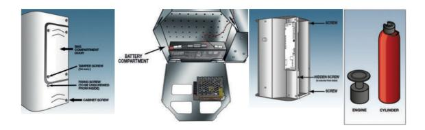
The screw in lower left part of cylinders compartment's door is longer than the others and its removal activates the tamper output. After the screw has been positioned correctly, the machine emits 4 beeps and deactivate tamper output.
