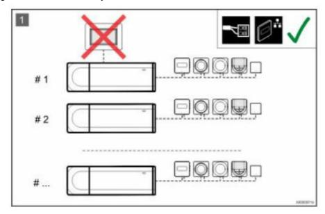
Connect and register thermostats, and system devices, to the controllers.
