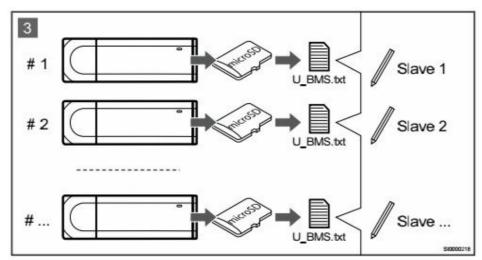
Edit the U\_BMS.txt file, on the controller microSD card, to setup
