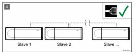
Connect the controllers to each other using the Base PRO controller system device bus.
