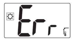
In "rS" mode, "Err" is displayed and the icon external sensor is shown.
