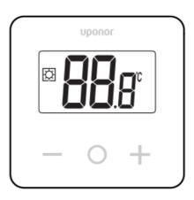
Uponor Base thermostat display T-27 230V (thermostat T-27) comes with a big LCD display and capacitive keys. The temperature is displayed in large digits for easy readability also from a distance. The capacitive keys and the front glass make cleaning of the front of the thermostat easy. A special electronics (triac) ensures that the thermostat is operating completely noiseless and provides the highest comfort in all rooms.
