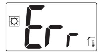
In "rt" mode, "Err" is displayed and the icon internal sensor is shown.
