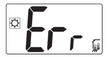
If the internal sensor fails, "Err" and the internal + floor sensor icons are shown.
