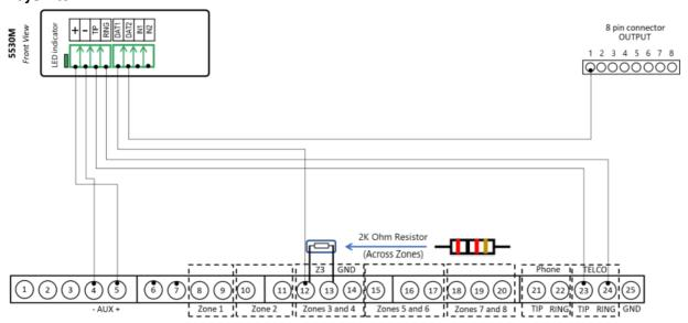
Programming the Honeywell Vista 20PSIA Alarm Panel via the Keypad Enable Contact ID reporting:
