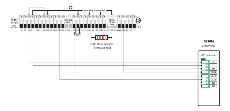
Wiring the 5530M communicators to DSC PC1616 / 1832 / 1864 for events reporting and remote control via keybus:
