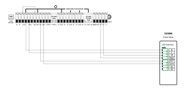
Wiring the 5530M with UDM to DSC PC1616 / 1832 / 1864 for remote upload/download.
