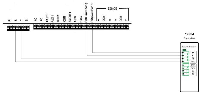
Wiring the 5530M with UDM to Interlogix NX-4 for remote upload/download
