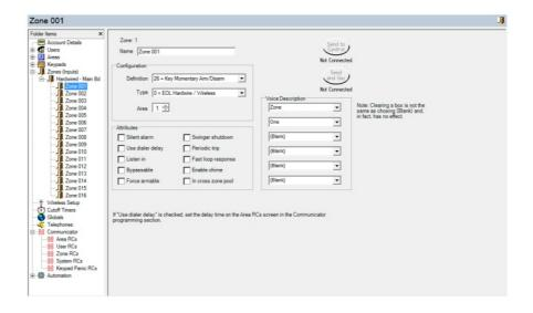
From ZONES, select Zone 1, Configure as Key Momentary ARM/DISARM, Type 0 = EOL, Area 1, Press Send to Control
