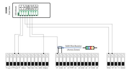
Wiring and Programming Uplink Communicators to DSC Power832/ PC5010 Wiring the 5530M communicators to DSC Power832/ PC5010 for remote control via keybus zone:
