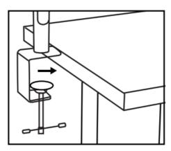
**Step 2:** Tighten the knob until the clamp is securely fastened to the edge of your desk.
