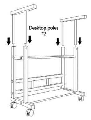
5. Mount the desktop pole on the desktop board with four 3cm flat head screws
