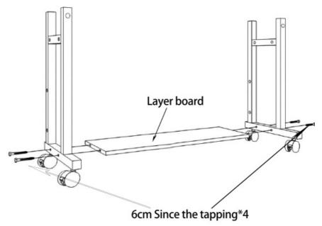
3. Tighten 4 x 6cm Since the tapping and 4 x 4cm flat head screws in the position shown in the picture
