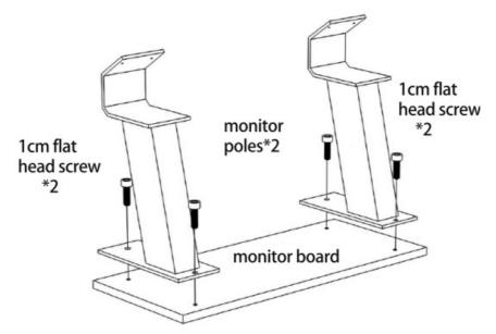
9. Insert the Monitor poles C-slot into the monitor board and tighten the 4 \* 1cm flat head screw
