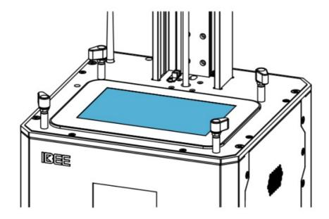
Put the Resin Tank back and lock it.
