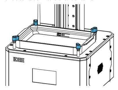
2. Check the Resin Tank, the film should be intact.
