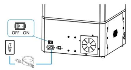
⚠ Make sure the Power Adapter is connected firmly to ensure stable power supply.
