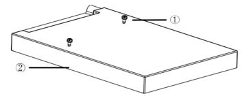
3. Slide the screws in the holes on the chassis bottom from A to B as illustrated and then tighten. Tighten two other screws to fasten the hard disk
