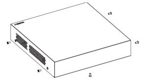
2. Insert the screws (e.g., ①) into the disk (②) and tighten halfway.
