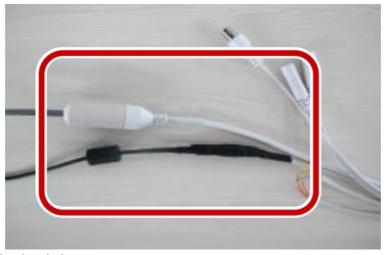
3. Protect other cables using insulating tapes.
