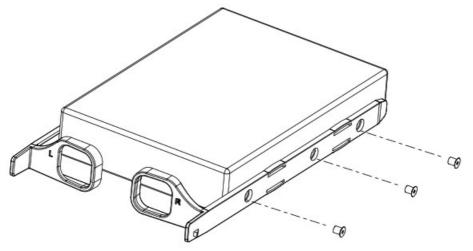
2. Press the latches on both sides, and then remove the front panel.
