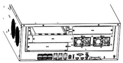
2. Align the service card with the slot, then push it gently into place.
