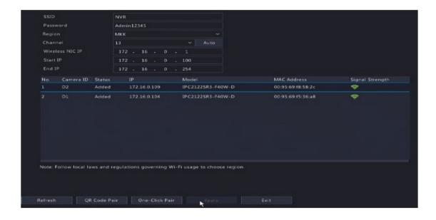
**CAUTION:** The NVR's wireless NIC IP must be in a different network segment from its LAN IP address.
