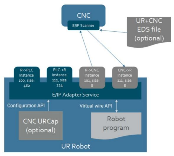
• Note that neither the CNC machine nor UR software needs to be modified, just configured.
