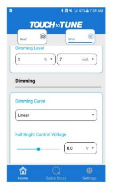
4. Selecting the "Basic Dimming" radio button disables the dimming curve and control voltages and only allows programming of the output current and dimming level.
