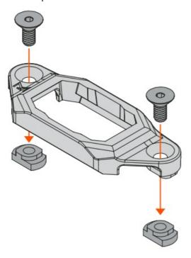
2. Insert the M-LOK® Screws through the AXON™ SL M-LOK® Mounting Kit Frame and thread partially into the M-LOK® nuts.
