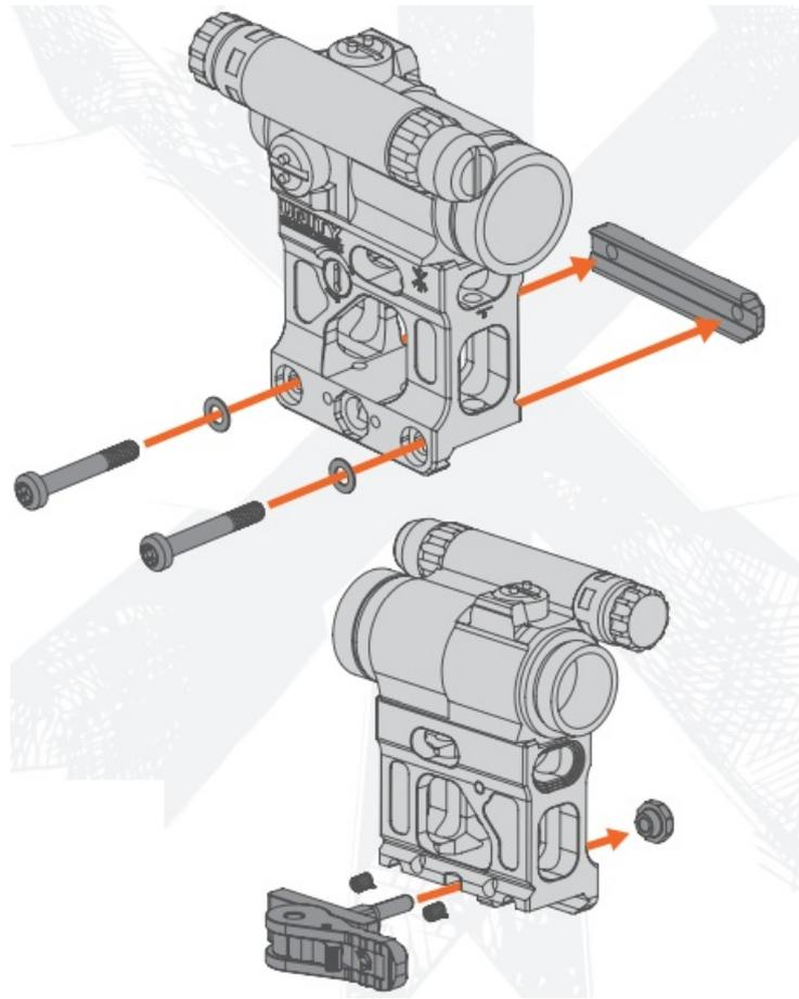
4. If using Standard Rail Grabber Mount clamp, install the mount on weapon. Secure screws using a T25 bit driver. Lightly snug all screws before applying final torque to any. TORQUE TO 35 IN-LBS.
