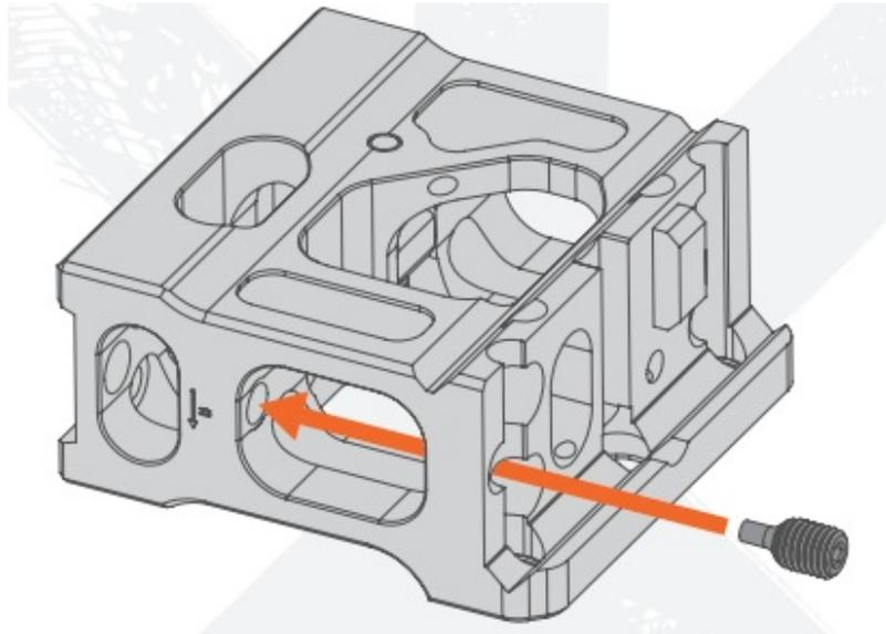
1. If using Front BUIS, thread into place through bottom of FAST Mount so tip of post is generally aligned with Rear BUIS. DO NOT USE THREAD LOCKER.
