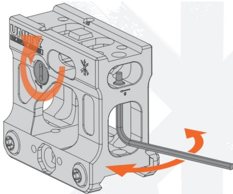
6. Windage adjustment of Rear BUIS is 0.5 MOA/click (with a 12.5" Sight Radius). If in conjunction with included Front BUIS, adjustment is 5 MOA/click. Windage adjustment can be made with Aimpoint adjustment tools or flat blade screwdriver.
