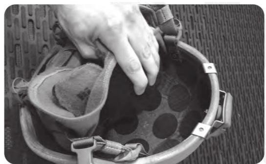
4. Remove CWLTM by grasping entire liner / pad assembly and slowly pulling it out of the shell. Take care to not tear fabric or stitching. Once removed, pull pads out of CWLTM and replace them in helmet.
