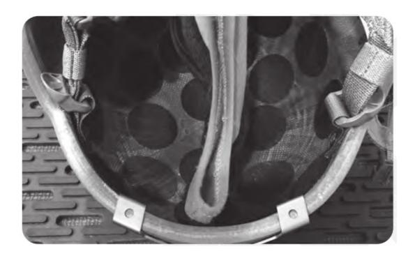
Keep CWLTM folded in half and align front center seam with center of helmet brim. Lower portion of CWL™ should extend below shell brim on most helmets. Align rear CWLTM seam with center of helmet rear edge. Carefully engage the "spine" of the CWLTM with Velcro running down the center of the helmet shell.
