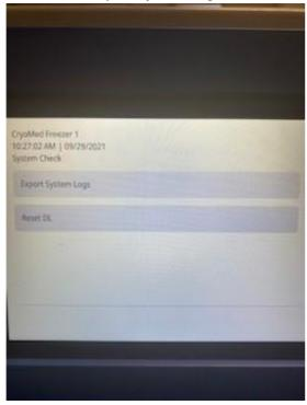
4. You will be prompted to insert a USB... "Please verify that a USB has been installed and has storage space". Insert an empty USB (8GB should be plenty of space) and click ok.
