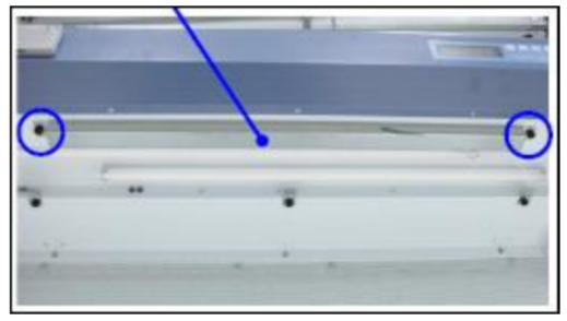
5. Please note the UV light resistant covers along with the UV lamp are recommended to be replaced every 1500 hours. See page 21, 37 in the operator's manual.
