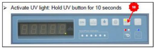
4. If the UV light still isn't functioning verify the UV bulb cover has been removed.
