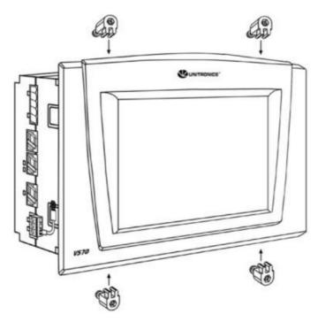
5. When properly mounted, the controller is squarely situated in the panel cut-out as shown below.
