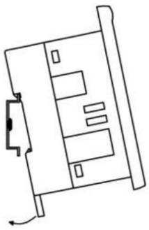
2. When properly mounted, the controller is squarely situated on the DIN-rail as shown in the figure to the right.
