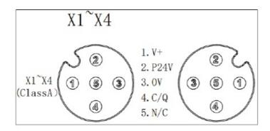
(When the IO-Link device is an input type, the 2 pins allow no wiring.
