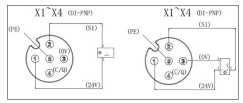
2. The PNP-type output signal, that is, the jack is connected to the actuator .
