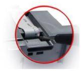
3. Gently remove the top of the device as shown.
