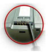
2. Taking care not to damage the cable, open the other side of the device by inserting the blade where shown below, then gently pushing up.
