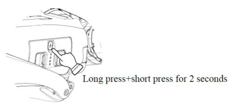
Please make sure that the robot turned off in a damping state, otherwise the robot will fall heavily on the ground after it is turn down and powered off, which may cause damage to the robot body and certain potential hidden dangers! If the power on fails, please check if the robot body is placed correctly.
