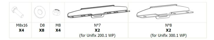
Connect both solar panels thanks to the connecting pieces  $N^{\circ}7$  and  $N^{\circ}8$  according to the models (Unifix 200.1WP and Unifix 300.1WP).
