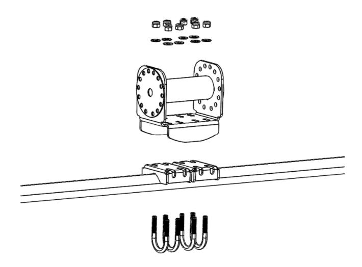
Fix both rotating pieces  $N^{\circ}4$  on the rotating basis  $N^{\circ}1$ .
