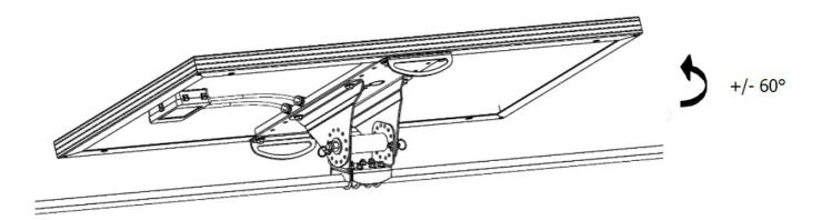
They can be fixed on tubes with a diameter from 20 to 45mm (minimum length of 100mm). With their galvanized steel structure and corrosion-resistant stainless-steel screws, they are perfectly suited for marine usage. Equipped with a multi-position tilting system, the Unifix mounting brackets optimize your electrical performances according to the chosen orientation.
