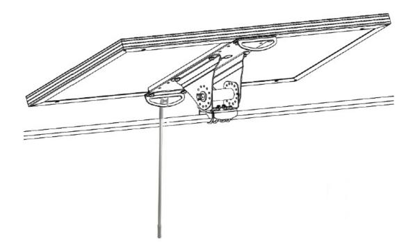
The angle can be maintained thanks to 2 ball pins and/or a rope system.
