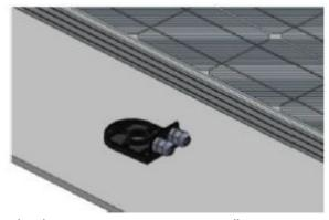
• Run the cables. Keep a sufficient length for wiring. Tighten the gland nuts to ensure a proper sealing.
