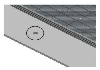
• Clean the fixing area with a degreaser. Do not use alcohol/white spirit.
