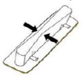
• Put glue on the indicated zone (in white on the image below), and place the roof-pass on the drilled area.
