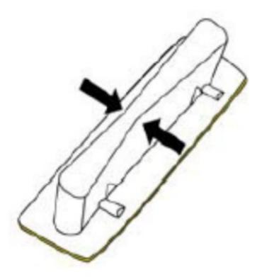
• Put the provided glue on the area indicated in white on the picture below, then put it over the drilling hole.
