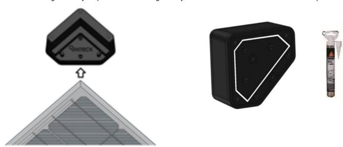
• Place the brackets on the previously marked surfaces. Press briefly down on the brackets.
