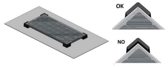
• Fix the 4 upper parts of the angles on the brackets using the flat washers, the lock washers and the cap nuts
