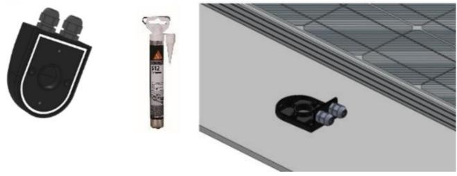
• Pass the cables as seen on the picture below. Keep a sufficient length for the connection. Tighten the nuts of the cable gland to ensure waterproofness
