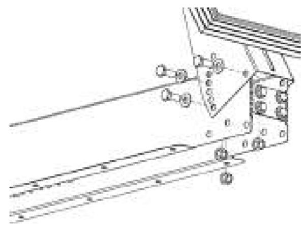
• Fix your bracket on a flat surface (hard floor or rigid wall) with 28 screws adapted to your surface (screws and dowels not supplied).
