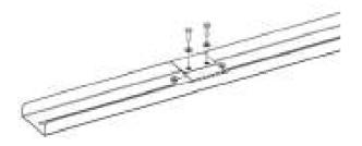
• Fold the two reinforcements by hand and screw it.
