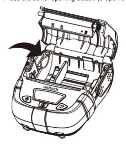
2. Load paper roln to the paper bin according 10 the direction as shown n the figure.
