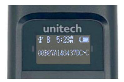
**Multiple read:** The terminal can read multiple tags that are under RF coverage upon each press. Keep pressing the Power / Trigger Key to read the tags that have not been read. The tags that had been read will not be read again, unless you release the button and press again.
