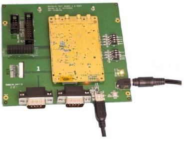
6. Insert the antenna connector into one of the four antenna ports of the RM300 Plus UHF RFID Reader Module. You can connect up to four antennas at the same time.
