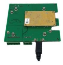
4. Insert the power connector into the power inlet on the interface board, and then plug the power adapter into an electrical socket.
