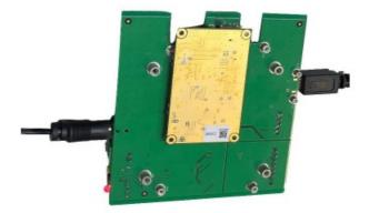
5. Insert the connector of the antenna into the antenna port of the RM100 UHF RFID Reader Module.
