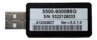
2. Plug the USB Dongle to a free USB port of a host computer. The MS852P is now ready to use.
