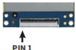
FPC connector (30Pin, Space between PINs 0.5mm)
