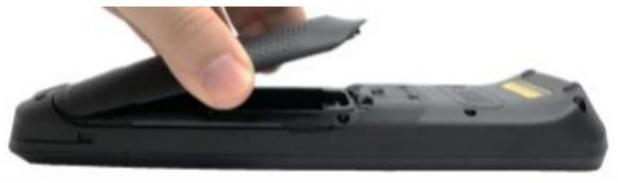
3. Press down the battery cover to secure in place. Make sure there is no gap between the device and the battery cover.
