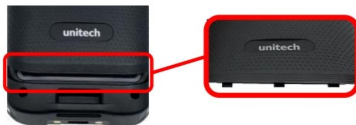
2. Insert the battery cover up to 45 degrees (45°) angle, from bottom to top.
