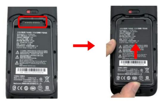
4. Press down 4. the battery to secure in place
