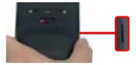
3. Align the battery with the battery compartment, then push forward until you hear a click sound
