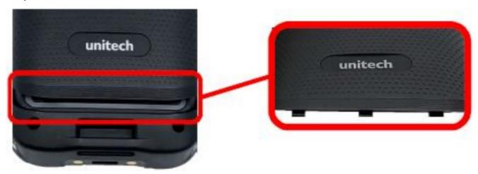
2. Insert the battery cover up to 45 degrees (45°) angle, from bottom to top.
