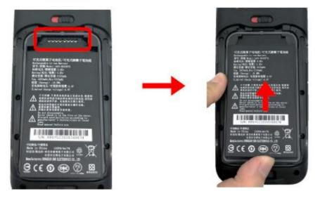
4. Press down the battery 4. to secure in place.
