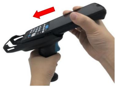
Slide the terminal into the gun grip, and make sure the terminal completely fits with the gun grip.
