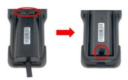
3. Align the hooks on the battery cover with the battery compartment, then press down the battery cover.
