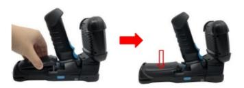
**4.** Push the battery lock to the right  $\stackrel{\triangle}{=}$  to secure the battery.
