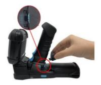
Grab and pull out the protective cover to remove.
