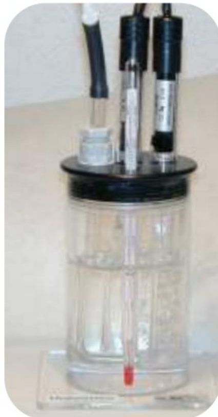
CAL300 with microsensors and bubbling with air.
