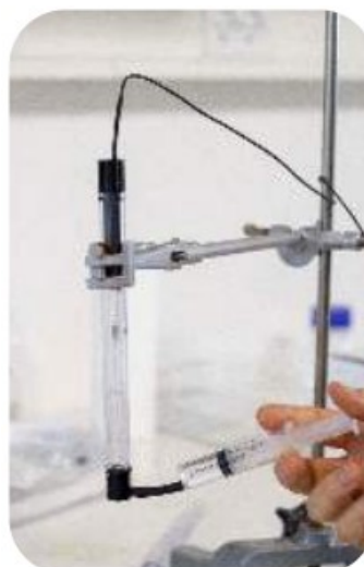
Injecting calibration liquid into protection tube using the calibration
