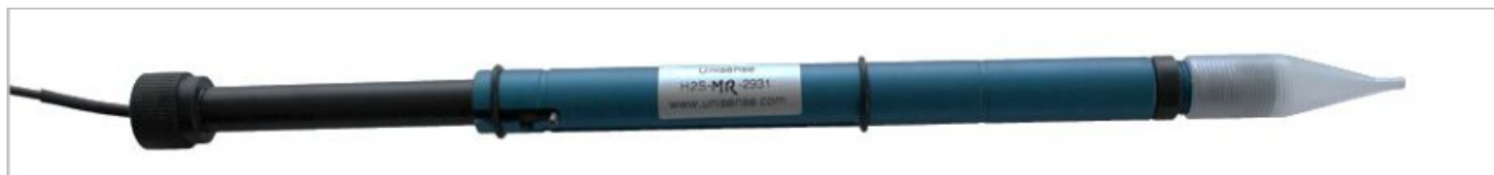
Figure 3: H2S sensor in the Micro respiration guide.
