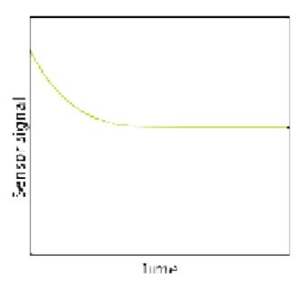
• A typical decrease in sensor signal over time for a sensor that has just been plugged in.
